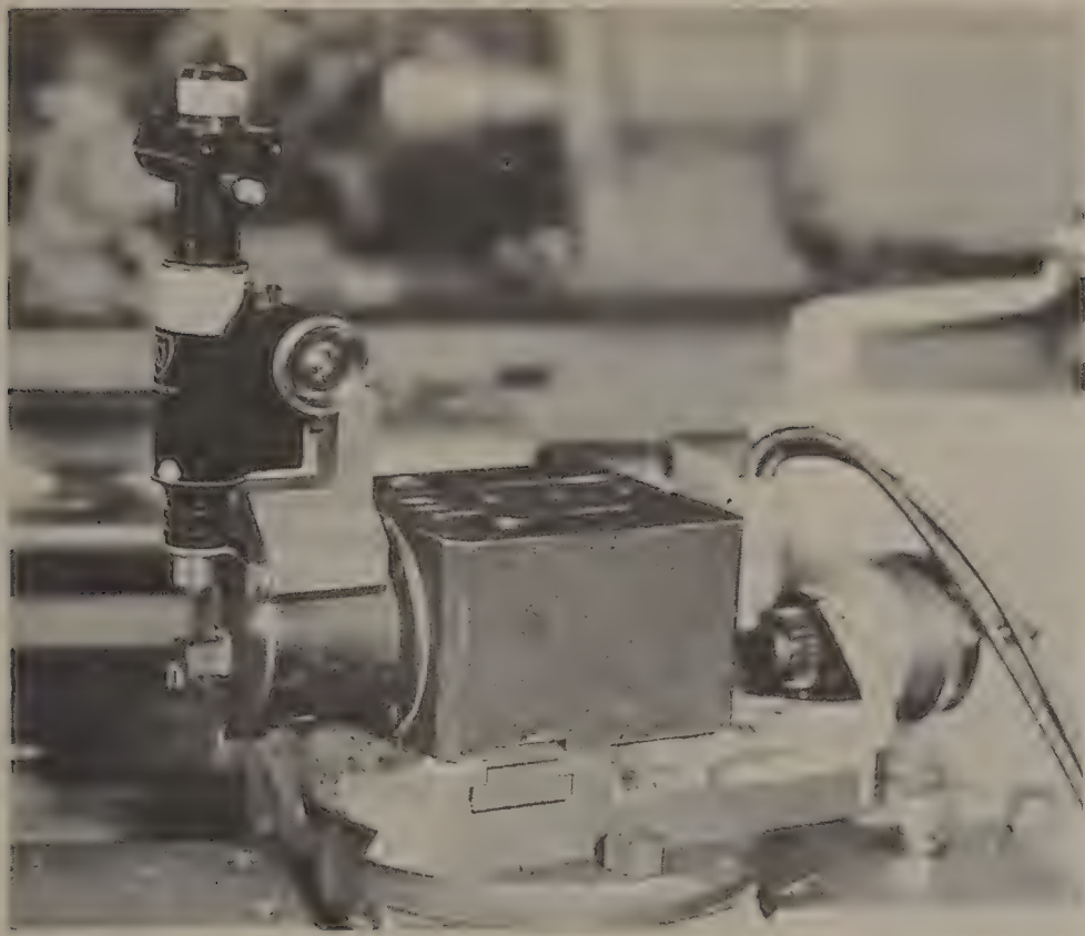
Fig. 35. Method used to examine tool faces in tool wear studies.
